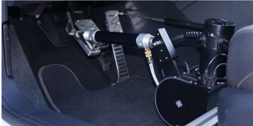
Illustration 18: Emergency Brake Robot integrated into Combined Pedal Robot CC800
