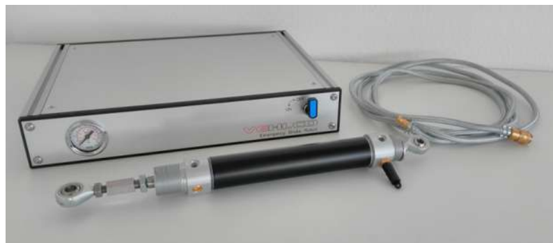
Illustration 17: Components of Emergency Brake Robot: Controller, Tube and Piston
