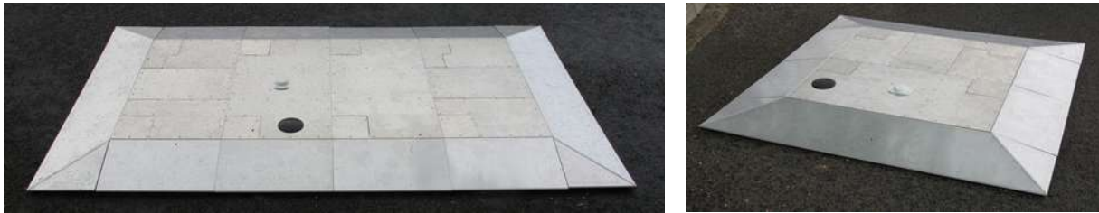
Illustration 30: Scalable Target Mover: For Vehicle Targets (left) and Bicycles/Pedestrians (right)
