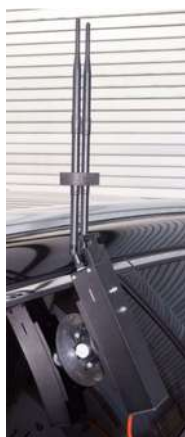
Illustration 37: Roof-/Window-Mounted IRC Access Point with High-Gain Antenna
