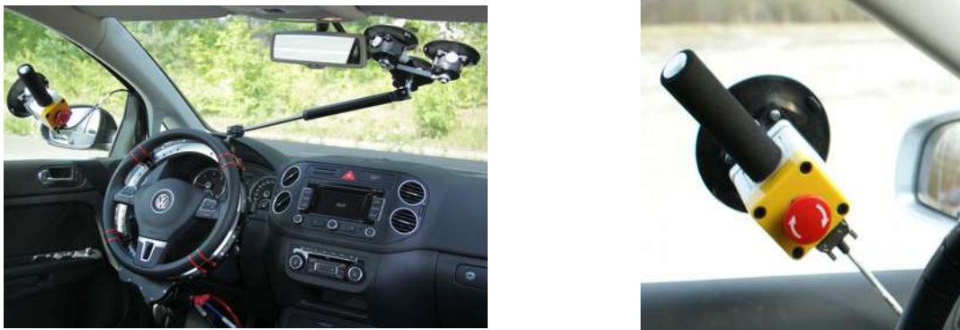
Illustration 4: Installation of the Steering Robot using Suction Mounting
