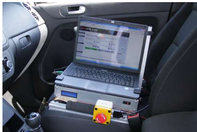
Illustration 20: The VEHICO Robot Controller installed on the Passenger Seat
