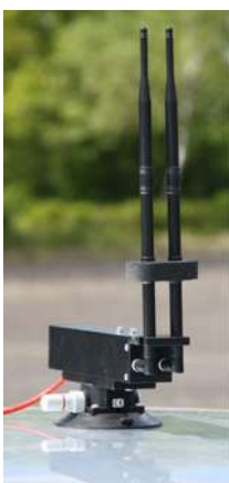
Illustration 37: Roof-/Window-Mounted IRC Access Point with High-Gain Antenna
