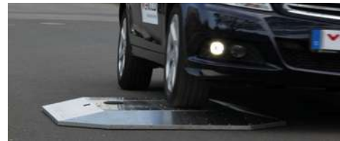
Illustration 33: Target Mover Withstands Dynamic Overrun
