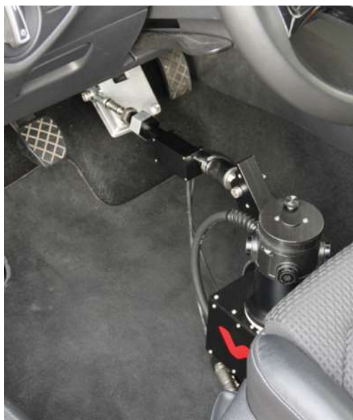
Illustration 13: Installation of Pedal Robot CP800 between Seat and Pedal
