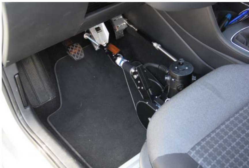
Illustration 15: Installation of Combined Pedal Robot CC800 between Seat and Pedal
