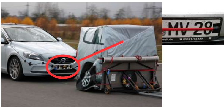
Illustration 27: Crash detection sensor mounted to front bumper
